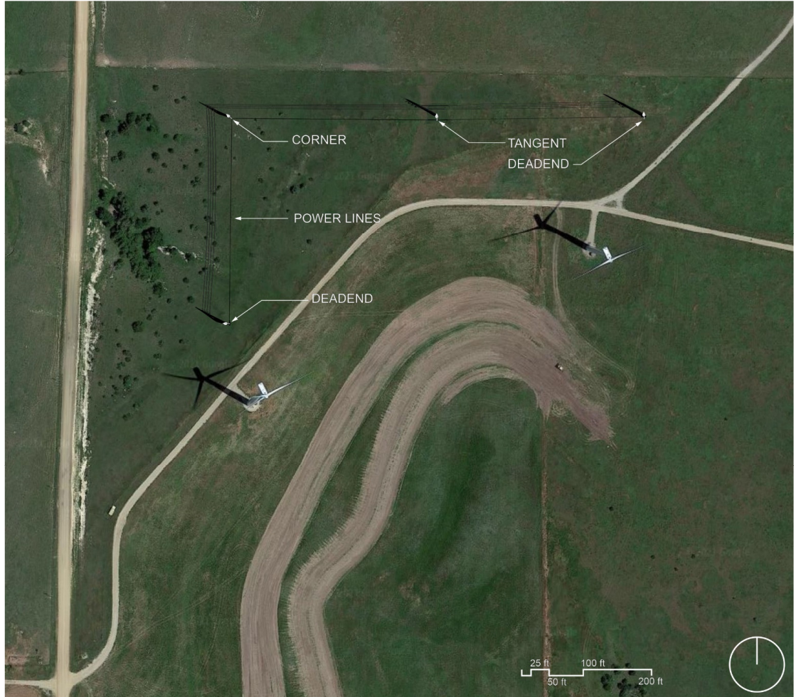
Planned Four-Pole Configuration in a wind farm in Kansas
