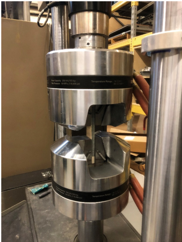
Fig. 6. Compression test set-up for spar cap material
