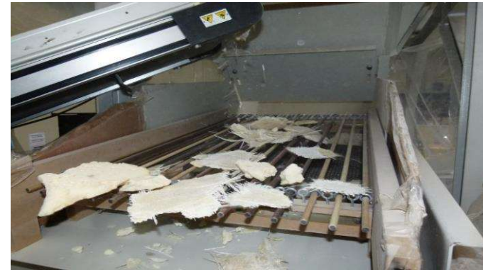
Cut GFRP composite waste Image: BRIO project Credit: Elhuyar Fundazioa
