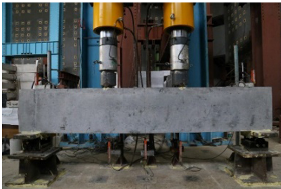
Fig. 12. Test set-up of the large-scale RC beam specimens.
