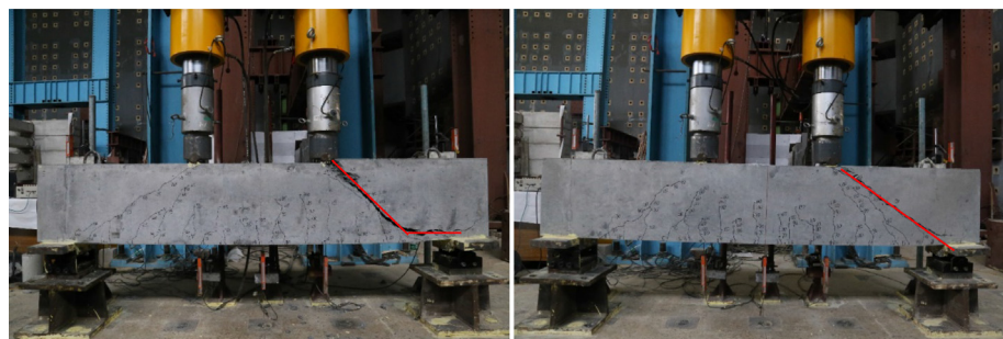
(a) Crack Pattern I
