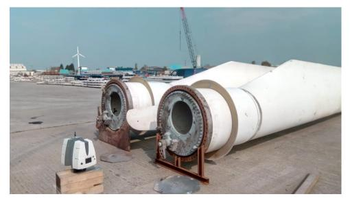
3D laser scanning of sample blades – Constructing a 'Digital Twin'
