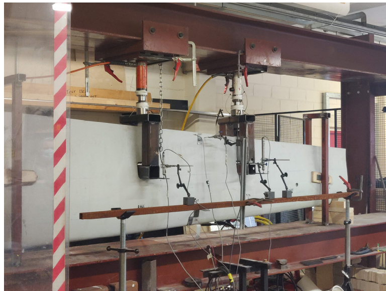
Figure 5. Structural testing of the LM 13.4 wind blade in the MTU structures laboratory.
