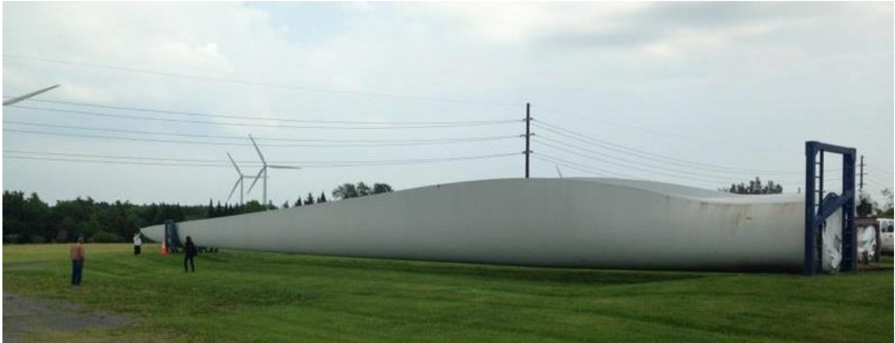
Vestas V82 from a 2004 1.65 MW turbine 40m long blade ~ 2.5m at max chord
